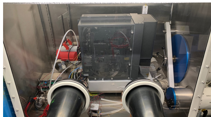
Phenom XL G2 Argon-Compatible Desktop SEM inside an argon-filled glove box.
