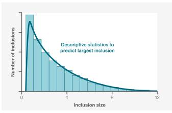
Combining the Phenom ParticleX Steel Desktop SEM with a statistical model, steel makers can predict the largest inclusions that are present according to ASTM E2283 standard practice for extreme value analysis.
