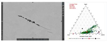
The Phenom ParticleX Steel Desktop SEM can be used for flexible SEM-EDS failure analysis during the day (left), while being set up for automatic and unattended inclusion analysis at night and on weekends (right).
